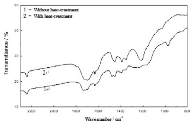
Figure 4 FTIR curves of the MAA/AN binary copolymer before and after the heat treatment.
